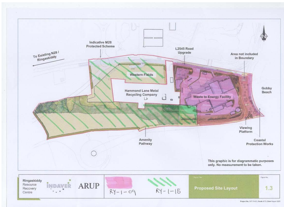
Figure 3 : Proposed site layout hand annotated by author to roughly indicate the two separate site zoning designations (Source of original :EIS Volume 3)
